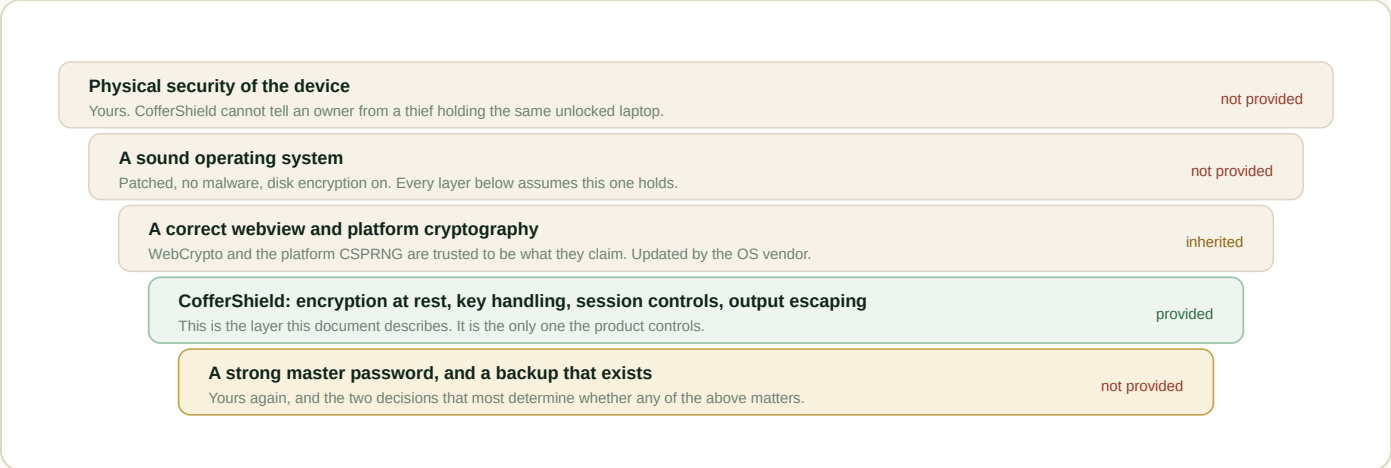
Figure 16 — Layers. Only the fourth band is CoffeShield's work. The outer bands are assumptions, and a failure in any of them defeats the middle.
